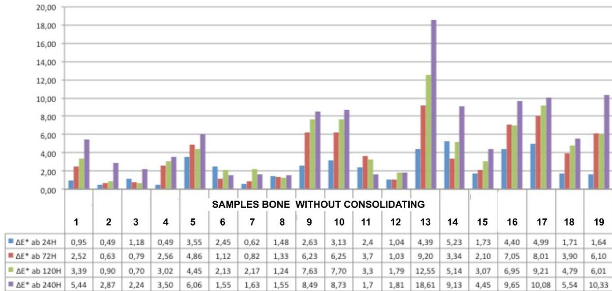
Figure AII-1 - Changes produced in bone material. Increments L\*, E00, C\* an h° after exposure of 240 h to UV radiation.
