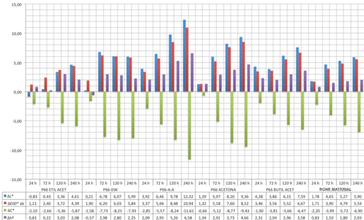
Figure AII-10 - Changes produced in areas treated with Paraloid™ B-66 on bone material. Increments L\*, E00, C\* an h° after exposure of 240 h to UV radiation.
