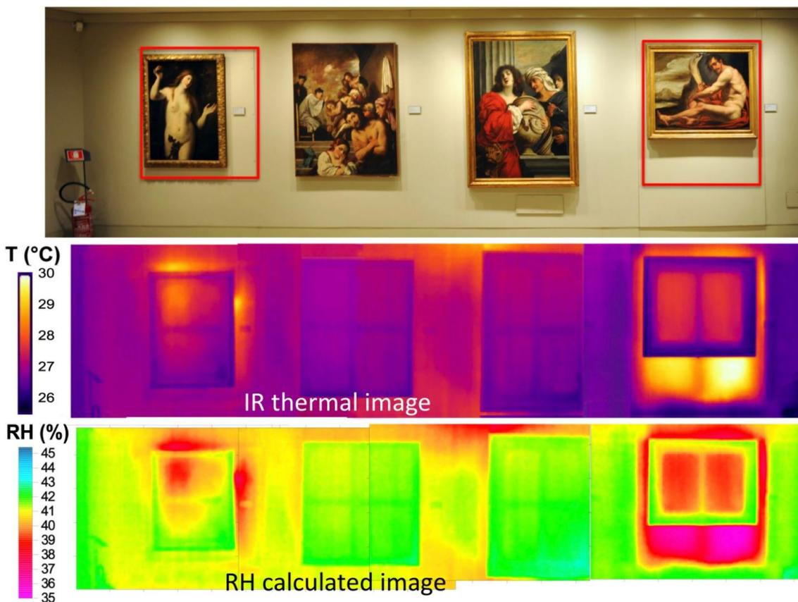
Figure 2 - View in visible light of paintings hung on a wall of a gallery; thermal image of the same wall taken with a thermocamera in the near infrared; image of the relative humidity at the interface between the air, the paintings and the wall, calculated using the temperature of the surfaces and the moisture content in the air.
