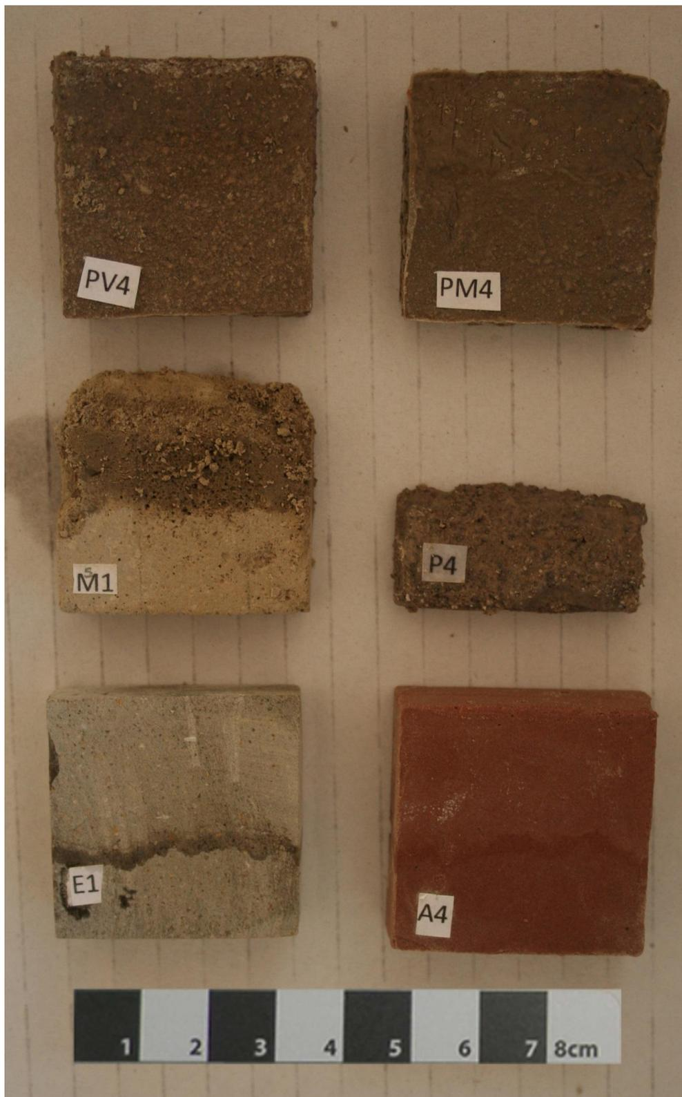
Figure 1 – Samples after the physical-mechanical characterization of working properties test, which shows reversibility after 30 minutes in ethanol.
