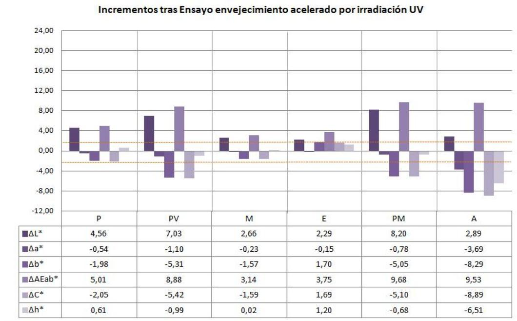
Figure 4 – Graphic of increase in (SCI)  $\Delta L^*$ ,  $\Delta a^*$ ,  $\Delta b^*$ ,  $\Delta AEab^*$ ,  $\Delta C^*$ ,  $\Delta h^*$  during the ultraviolet radiation accelerated artificial aging test after processing colorimetric data.
