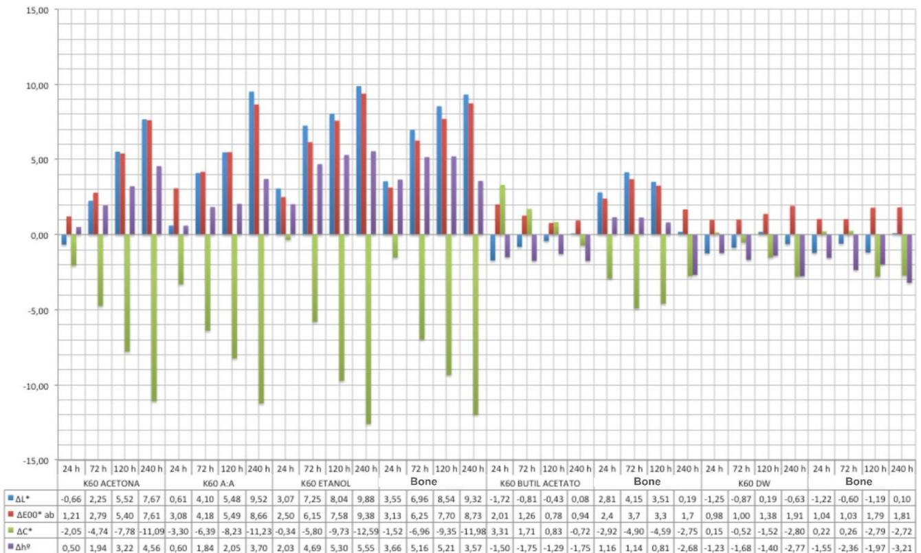
Figure AII-6 - Changes produced in areas treated with K60 on bone material. Increments L\*, E00, C\* an h° after exposure of 240 h to UV radiation.
