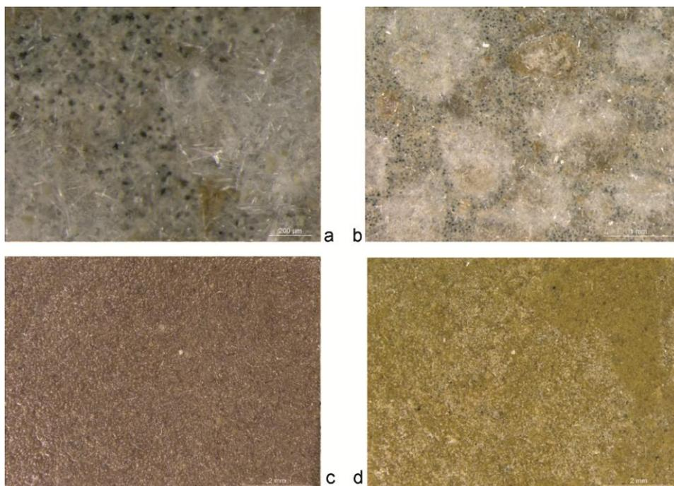
Figure 6 - A,B) (x16) possible salt efflorescence in Epo150<sup>®</sup> filler after SO<sub>2</sub> saturated atmosphere accelerated artificial aging test. C,D) Araldit SV427<sup>®</sup> before and after SO<sub>2</sub> saturated atmosphere accelerated artificial aging test where what seems to be salt efflorescence appears in the image taken after the test.
