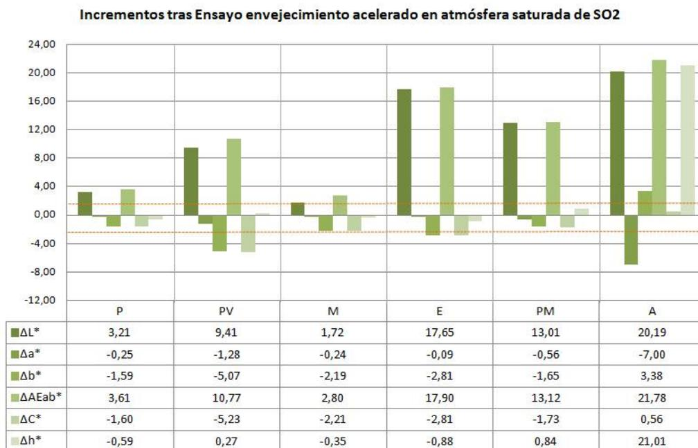
Figure 5 – Graphic of increases (SCI)  $\Delta L^*$ ,  $\Delta a^*$ ,  $\Delta b^*$ ,  $\Delta AEab^*$ ,  $\Delta C^*$ ,  $\Delta h^*$  after SO<sub>2</sub> saturated atmosphere accelerated artificial aging test after processing colorimetric data.
