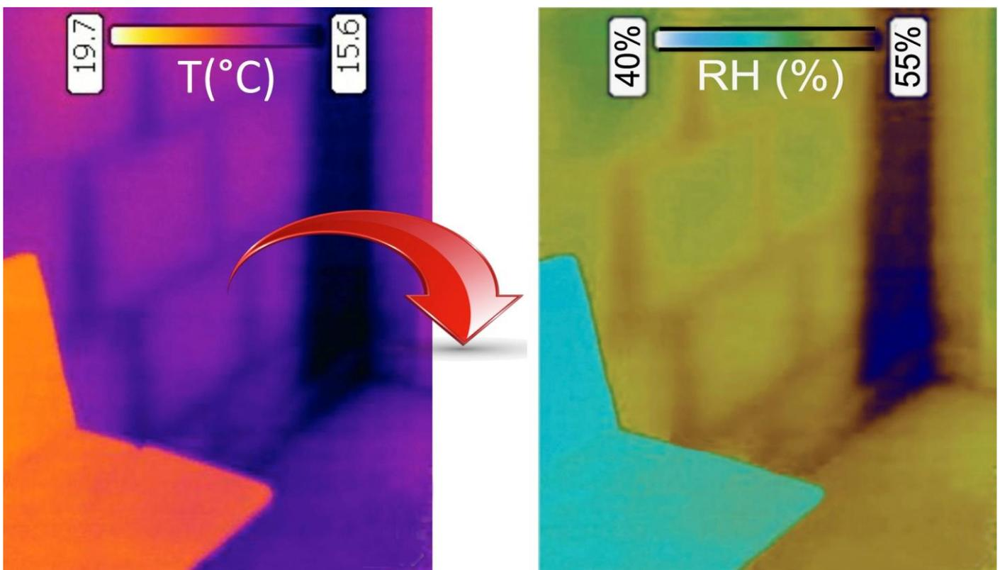
Figure 3 - Thermal image of a cold corner in a heated room in winter, taken with a thermocamera in the near infrared; image of the relative humidity at the interface between the air and the wall, calculated using the temperature of the surfaces and the moisture content in air. The arrow shows the internal air circulation. A warmer bench (at indoor air temperature) is visible on the left side.
