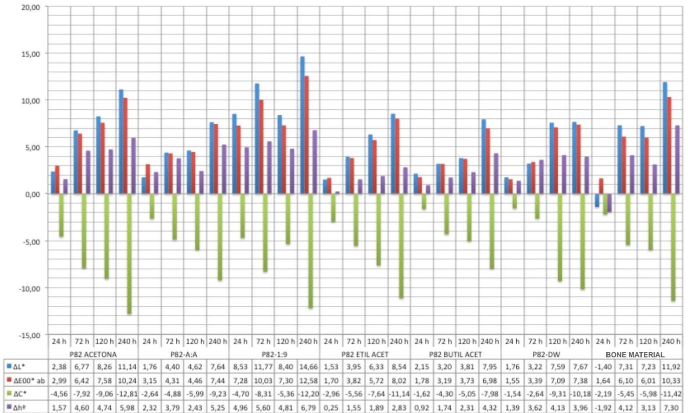
Figure AII-11 - Changes produced in areas treated with Paraloid™ B-82 on bone material. Increments L\*, E00, C\* and h° after exposure of 240 h to UV radiation.
