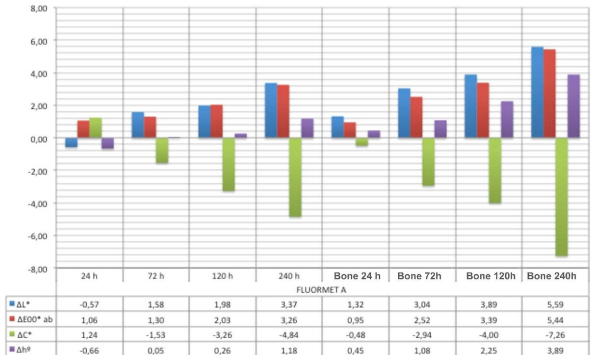
Figure AII-2 - Changes produced in areas treated with Fluoline-A on bone material. Increments L\*, E00, C\* an h° after exposure of 240 h to UV radiation.
