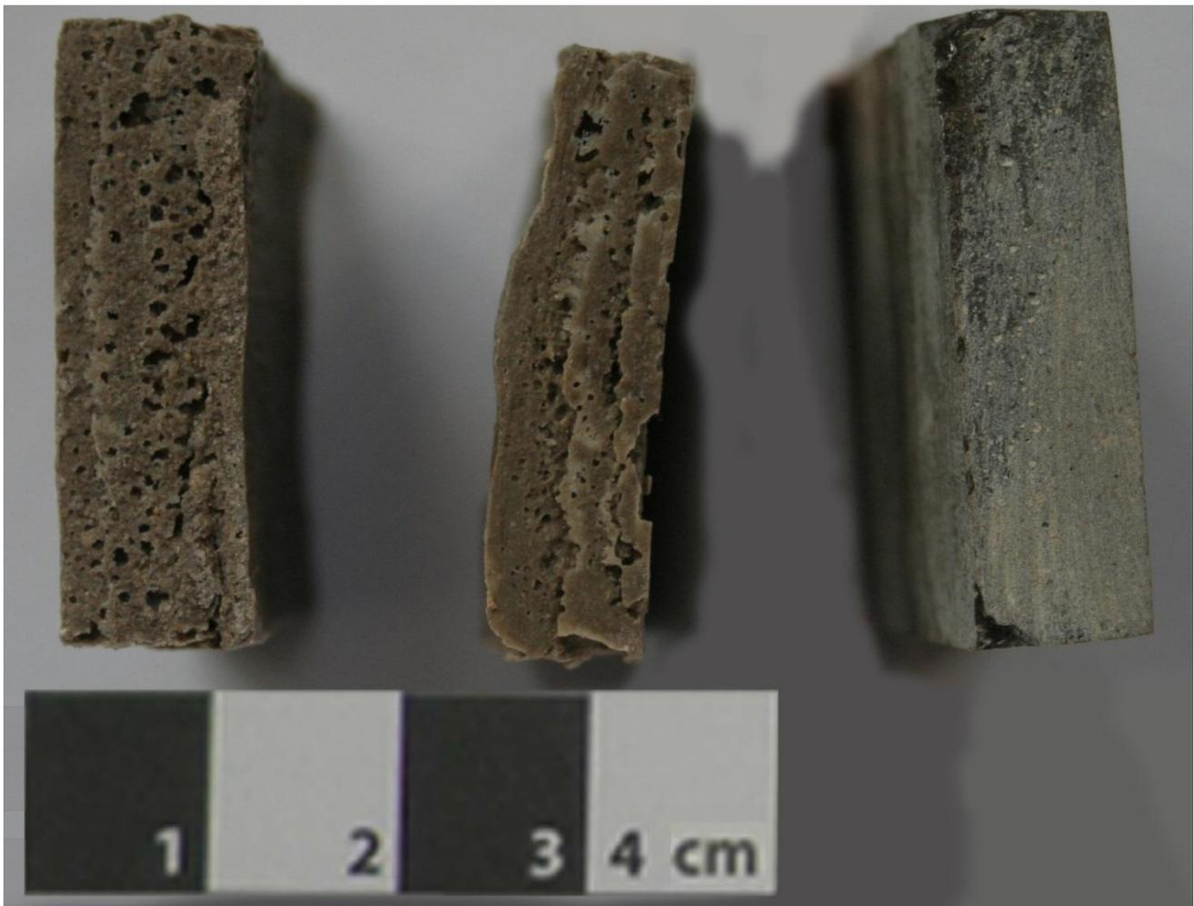
Figure 2 – Detail of strata drying in PVAs gap fillers compared to Paraloid B72<sup>®</sup> gap fillers.
