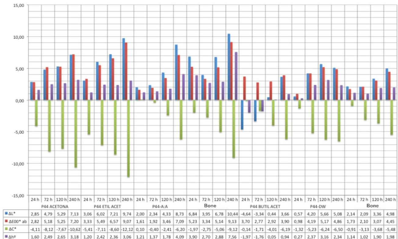
Figure AII-8 - Changes produced in areas treated with Paraloid™ B-44 on bone material. Increments L\*, E00, C\* and hº after exposure of 240 h to UV radiation.
