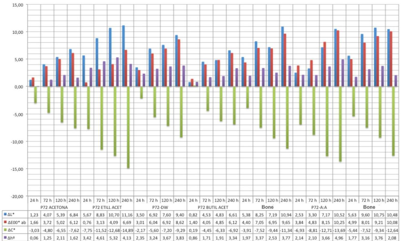
Figure AII-9 - Changes produced in areas treated with Paraloid™ B-72 on bone material. Increments L\*, E00, C\* an h° after exposure of 240 h to UV radiation.
