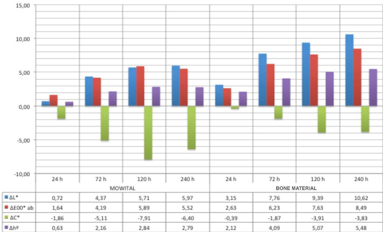
Figure AII-5 - Changes produced in areas treated with Mowital® on bone material. Increments L\*, E00, C\* an h° after exposure of 240 h to UV radiation.
