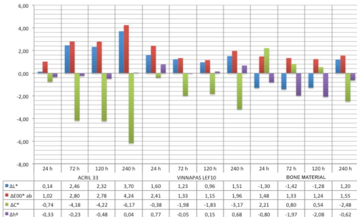
Figure AII-4 - Changes produced in areas treated with emulsions resins (acril-33 and Vinnapas® LEF10) on bone material. Increments L\*, E00, C\* an h° after exposure of 240 h to UV radiation.
