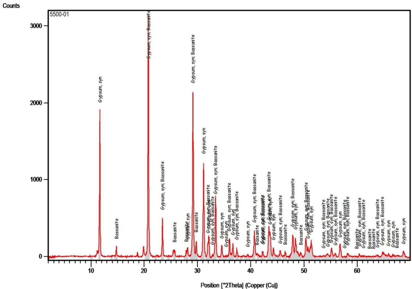
Figure 5 - X-ray powder diffraction (XRD) diagram of material analyzed.
