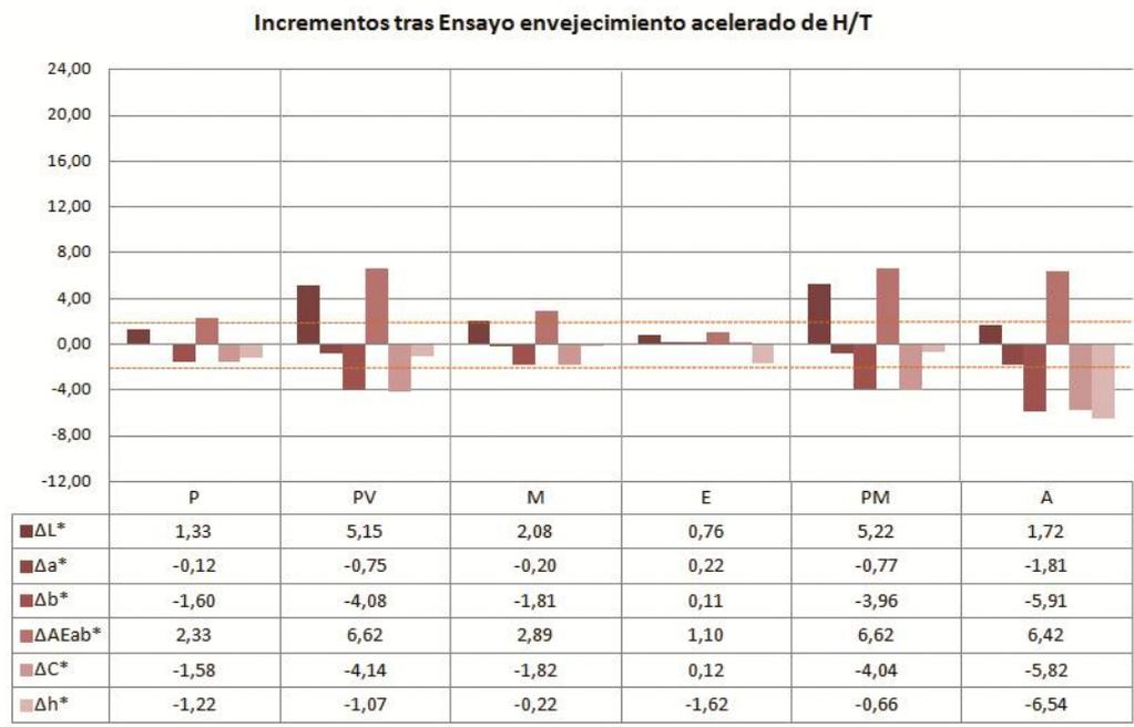
Figure 8 - Graphic of increases (SCI) ΔL\*, Δa\*, Δb\*, ΔAEab\*, ΔC\*, Δh\* after the humidity and temperature accelerated artificial aging test after processing colorimetric data.
