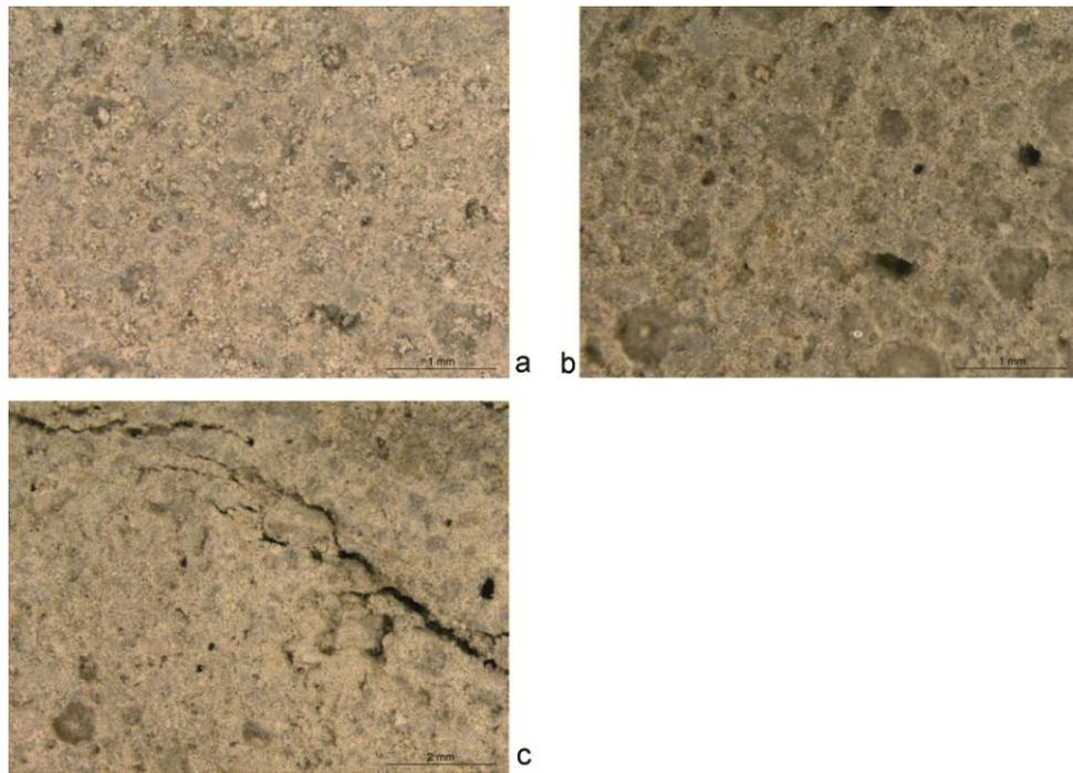
Figure 7 - A) (16x) shows the sample before the test. B,C) higher porosity and cracks after SO<sub>2</sub> saturated atmosphere accelerated artificial aging test in the Mowital B60HH® filler.
